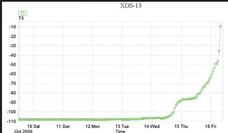
Test 3 Using 135# dry ice, Texas Foam XDS-13 256 hours to -20 C
